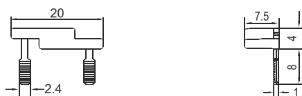
S1D-B1, 10A @ 250 VAC, 1 Way Bridge for Coil
